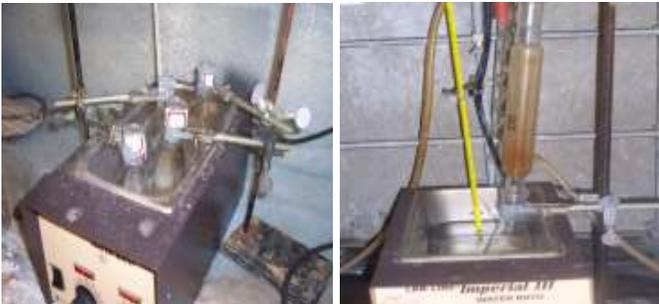
**Figure 5.** Fiber Volume Fraction Test Setup
