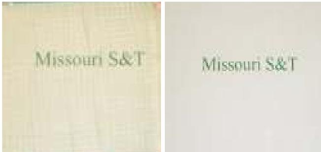
**Figure 4.** Transparent Composite (Left) vs. Glass Plate (Right)
